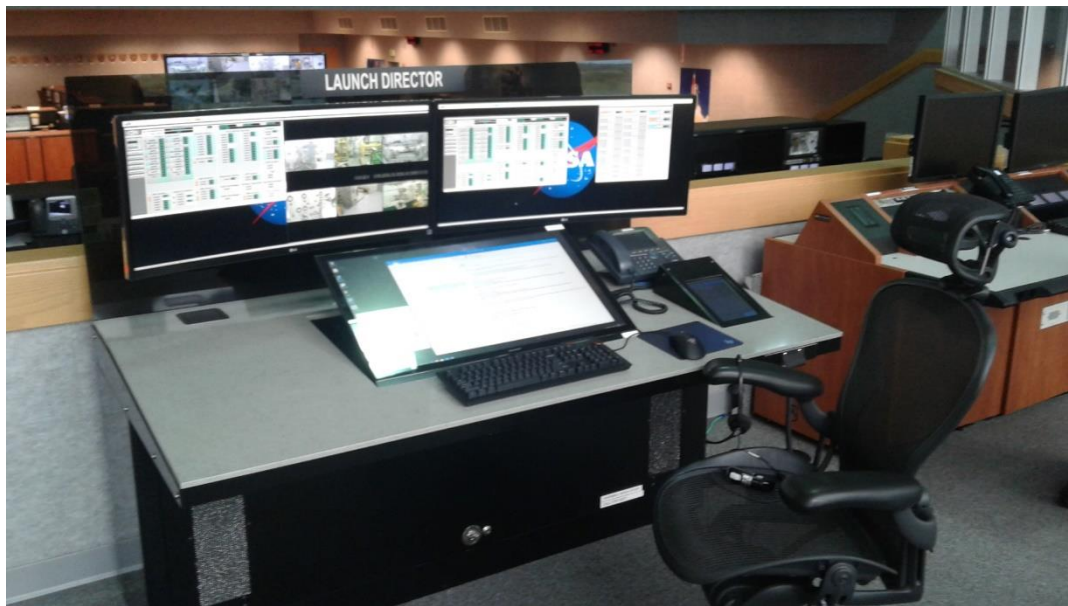
Image 1. Operational Launch Director Console Pictured above is the completed LDC, including its 2 ultra-wide monitors, adjustable touchscreen, telephone, and OIS-M unit.
