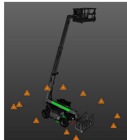
Figure 7. Man lift scan data in RealWorks with both the extended and retracted lift point clouds. The green plane was fitted to the lift arm and used to create a user-defined coordinate system.
