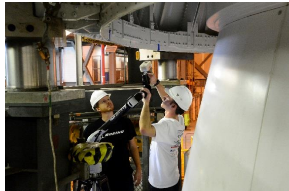
Figure 9. The author using the ROMER arm under the SRB aft skirt. On the left is Rich Overleese and behind the camera is Devin Swanson, who both helped me tremendously during the internship.
