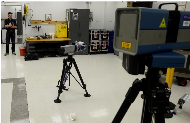
Figure 4. The laser tracker is in the middle surrounded by spherical white scan targets. I was standing out of the way as the Surphaser on the right was scanning. Behind the camera is Devin Swanson who helped me with this scan.
