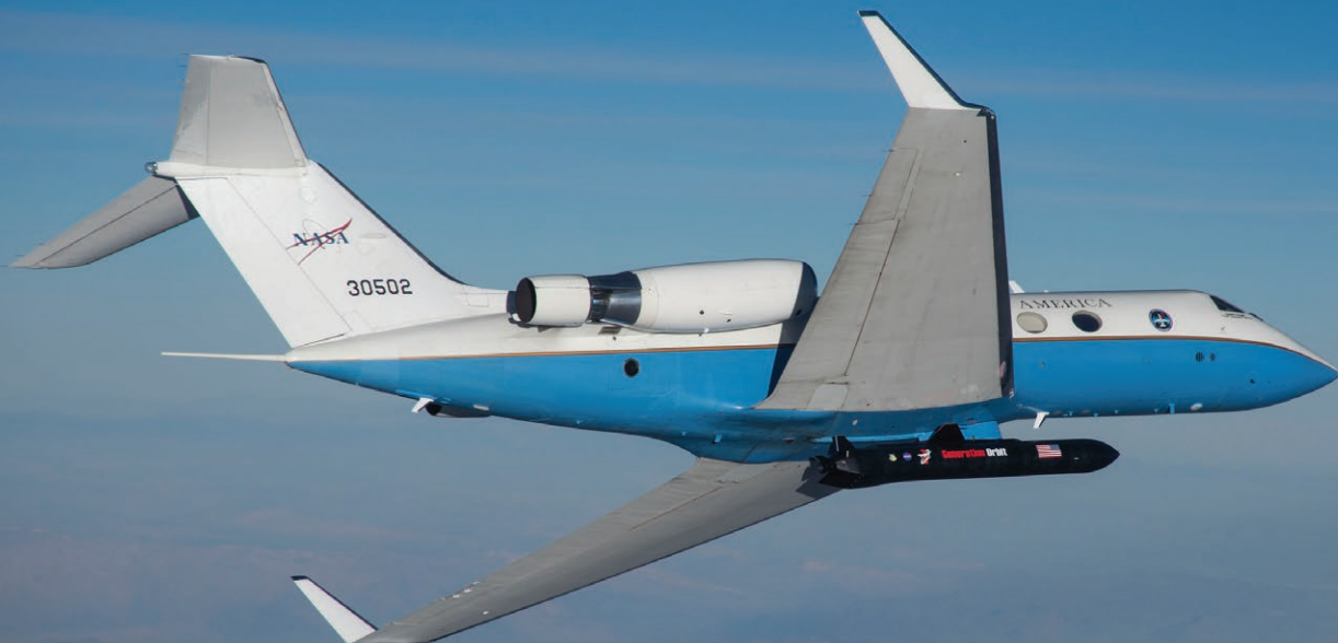
NASA's C-20A, with Generation Orbit's hypersonic pod attached, undergoes flight test over Armstrong.
