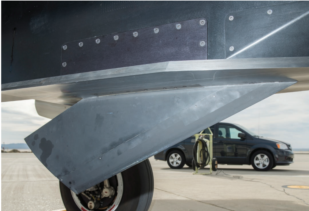
NASA's F-15 research testbed will expose the swept wing laminar flow test article to speeds up to Mach 2, matching conditions presented during wind tunnel tests.
