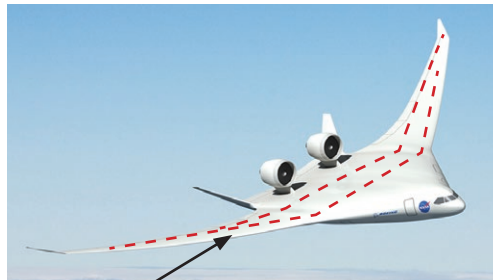
Installed strain sensors
