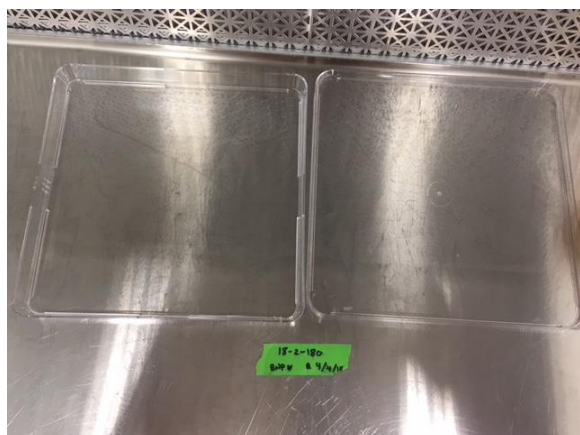
Image 2. Solutions poured into 8” x 8” plates to dry under a laminar flow hood.
