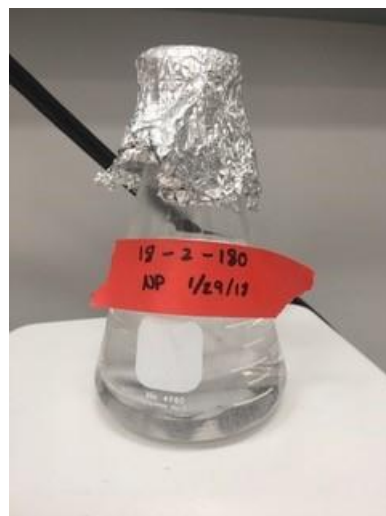
Image 1. A film solution clear of pullulan powder clumps after five hours of stirring.
