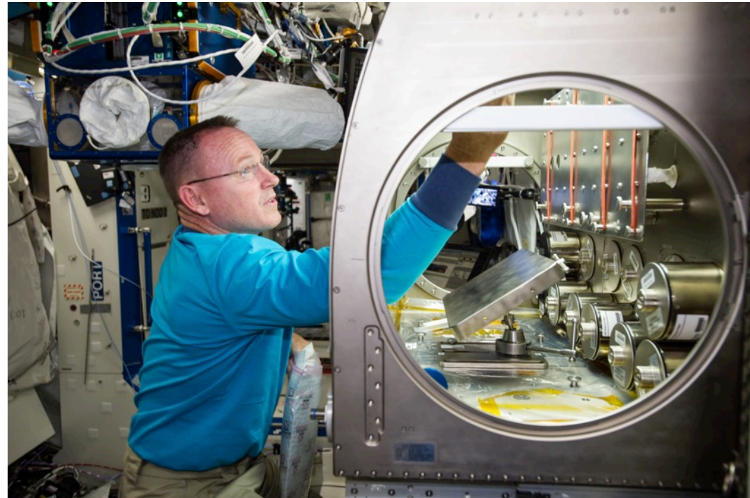
NASA astronaut Barry "Butch" Wilmore setting up the Rodent Research-1 hardware in the Microgravity Science Glovebox aboard the International Space Station.
