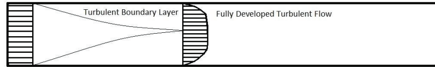
Fully developed turbulent pipe flow schematic
