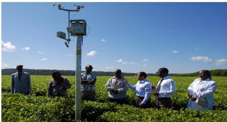
NASA low cost Wireless Sensor Network for in situ temperature, humidity, wind and rainfall Data collection for Frost monitoring calibration
