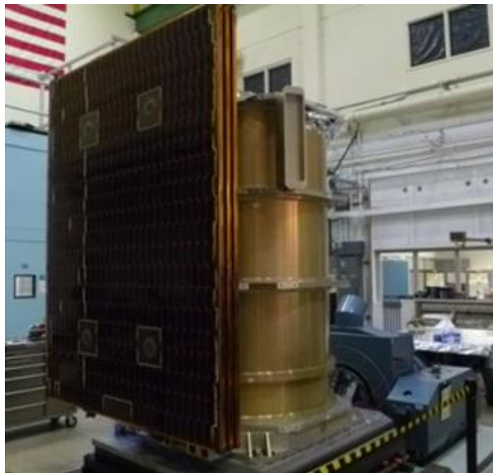
Figure 17. Solar Array Subsystem Vibration Testing
