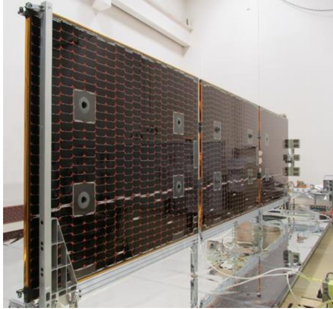
Figure 15. Deployed Array on Air Bearing Support Equipment
