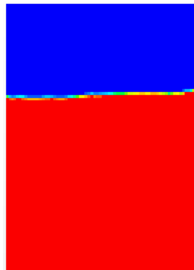
Figure 24. 564k polyhedral mesh liquid volume fraction (bottom section is liquid)
