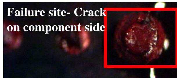
(b) Failure on component side
