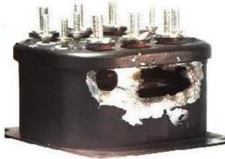
Failed relay due to tin vapor arcing
