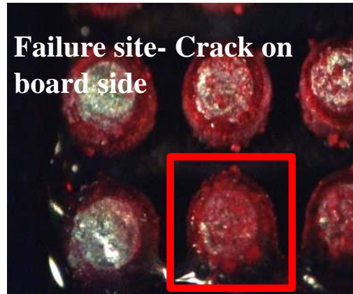
(a) Failure on board side
