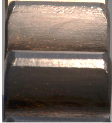
Figure 8 – Red-brown coloration noted after 77 days exposure to humid air
