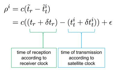
• Transmission and receive times each expressed as a sum of the "true" time (i.e., the time according to a common time standard, such as GPST) plus an unknown bias
