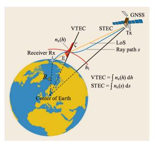
Geometry of zenith TEC (vertical TEC, VTEC) and slant TEC (STEC) [13]
