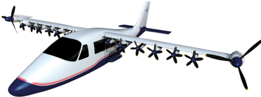
Figure 2. The X-57 Maxwell DEP aircraft. The Tecnam P2006T fuselage, vertical tail and stabilator with the DEP wing system that includes the wingtip propulsors and the DEP high-lift motors.
