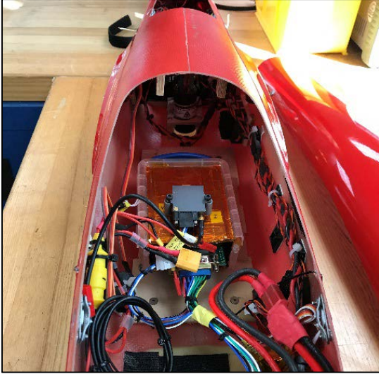
Figure 15 – Safeguard installation in Tempest-1 aircraft.
