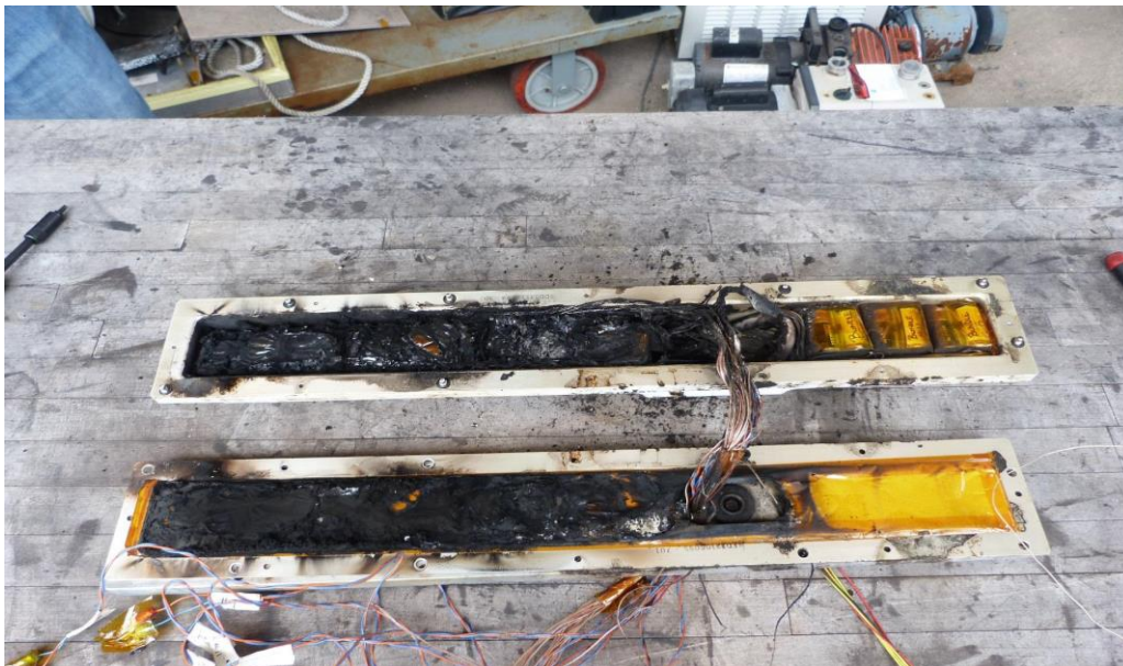
Figure 7.4-27. Test #4 Post-test Image of Open Battery Pack
