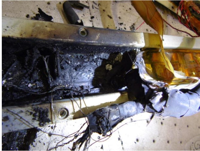
a) Close up of 4S bundle cavity and demarcation line between 4S bundle and 10S bundle.
