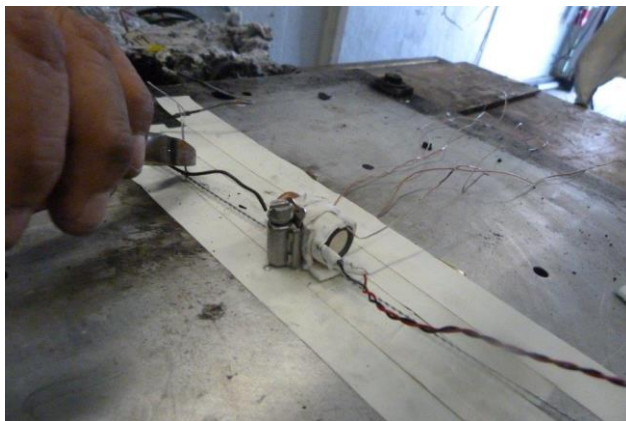
Figure 7.3-8. Cell on a 49 °C Hotplate Being Prepared for Testing
