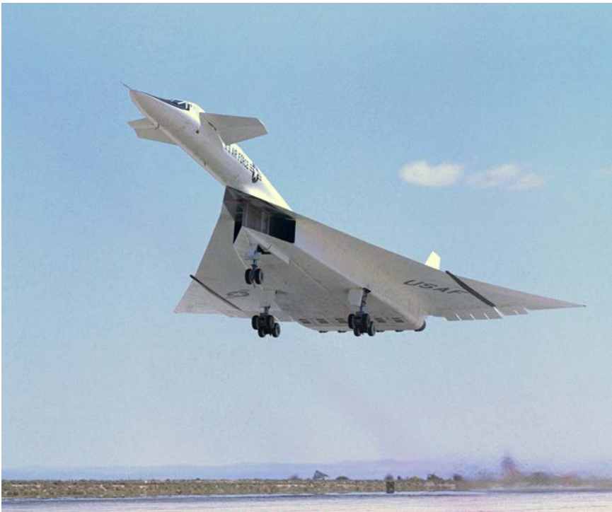
Figure 2-3. The XB-70 was the world's largest experimental aircraft when the Air Force and NASA partnered to use the canceled bomber as a flying laboratory to generate data for future supersonic aircraft. The controllable internal geometry of the inlets maintained efficient airflow to the six YJ93 turbojets. (NASA)
