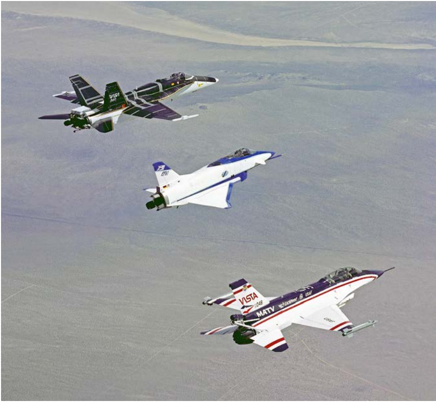
Figure 5-10. Shown are the F/A-18 HARV, the X-31, and the F-16 MATV, all thrust-vectoring research aircraft. (NASA)
