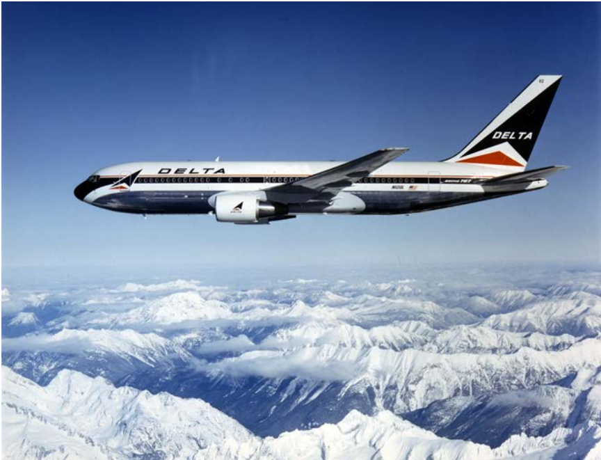
Figure 4-4. Pictured is a Boeing 767 with Pratt & Whitney PW4000 turbofans in the mid-1990s. (Delta Air Lines)
