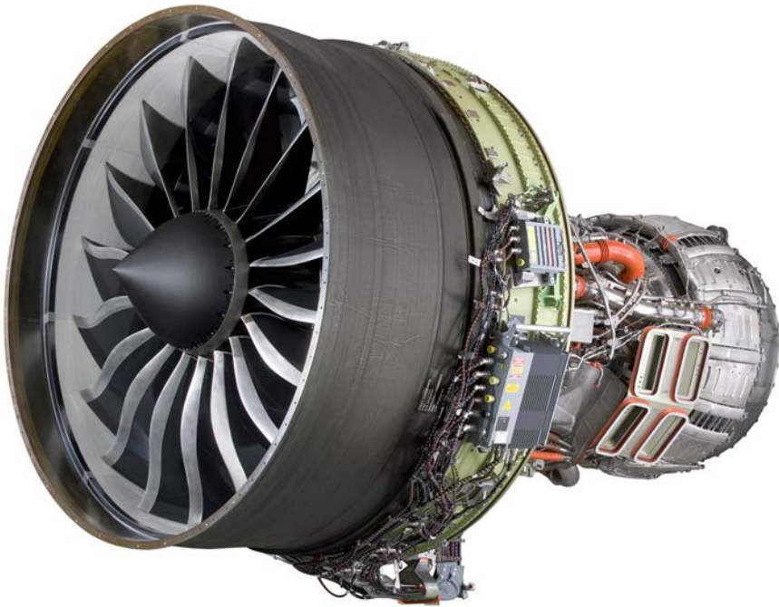
Figure 6-1. The advanced fan blades and composite fan casing of the GE GENx-2B engine reflect NASA's pioneering work. (General Electric)
