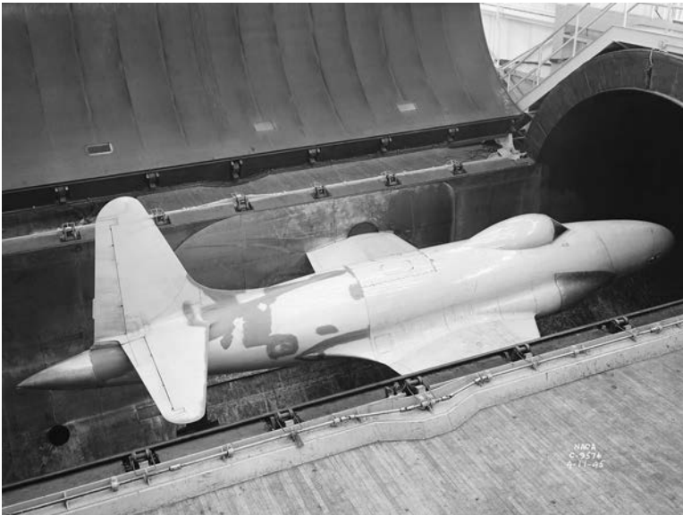
Figure 1-9. The NACA created the Altitude Wind Tunnel to test full-scale piston engines and propellers in simulated altitude conditions. The first tests of a turbojet engine took place in February 1944. During the spring of 1945, researchers installed a full-size Lockheed YP-80A Shooting Star fuselage with a GE I-40 engine for high-altitude evaluation. The tests led to data that predicted the engine thrust at all altitudes, which contributed to the operational success of America's first practical jet fighter. (NASA)
