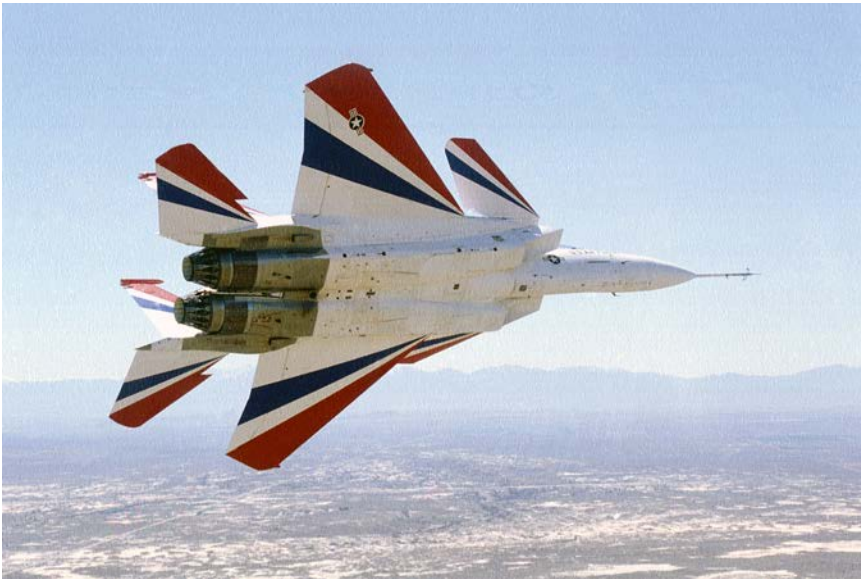
Figure 5-9. The Pratt & Whitney pitch-yaw balance beam nozzle system enabled vectoring horizontally (yaw) and vertically (pitch). The ACTIVE program achieved the first supersonic yaw-vectoring flight on April 24, 1996. (NASA)
