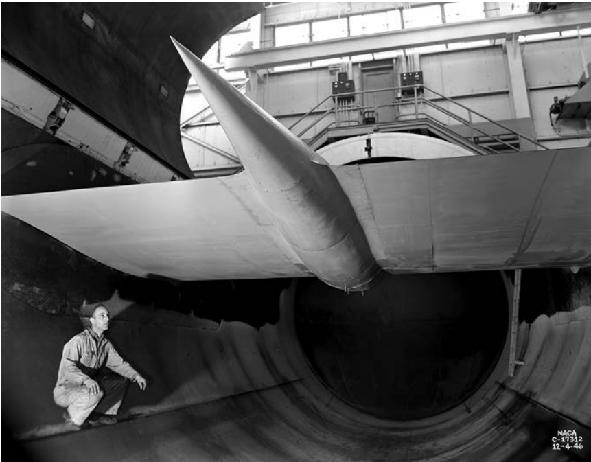
Figure 1-12. Besides the turbojet, NACA researchers in Cleveland, OH, investigated other new propulsion technologies. The first turboprop flown in the United States, the GE TG-100A, underwent tests in a streamlined nacelle to determine the performance characteristics of the compressor and turbine in the Altitude Wind Tunnel in late 1946. (NASA)
