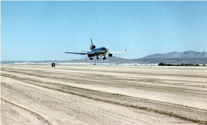
Figure 5-7. In August 1995, Gordon Fullerton brings the MD-11 in for the first PCA landing of an airliner. (NASA)
