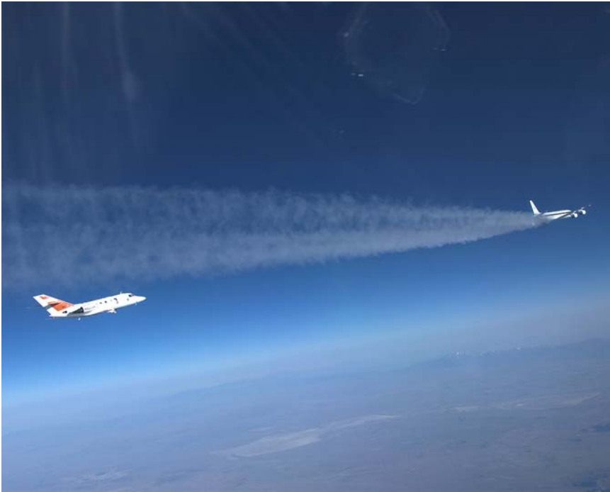
Figure 7-6. The researchers of the ACCESS project used Langley’s heavily instrumented HU-25 Falcon to measure the chemical composition of the DC-8 Airborne Science Laboratory’s exhaust contrail generated by a 50-50 mix of conventional JP-8 jet fuel and a plant-derived biofuel. (NASA/Lori Losey)
