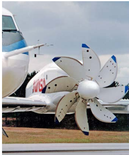
Figure 4-7. The propfan on the Gulfstream II. (NASA)
