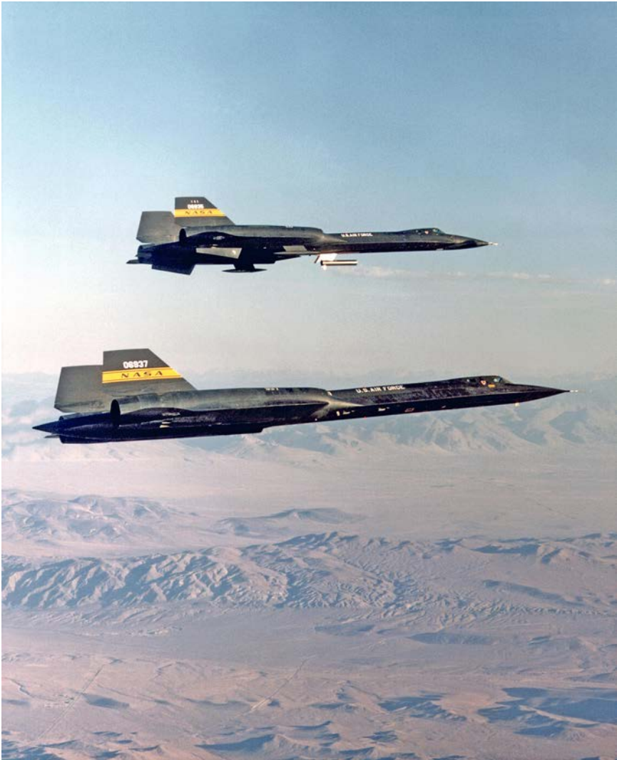
NASA maintained an active research program with its Lockheed YF-12 Blackbirds from 1967 to 1979, which included propulsion-focused investigations. The Blackbird at top carries the experimental "coldwall" heat transfer pod on a pylon beneath the fuselage in 1975. (NASA)
