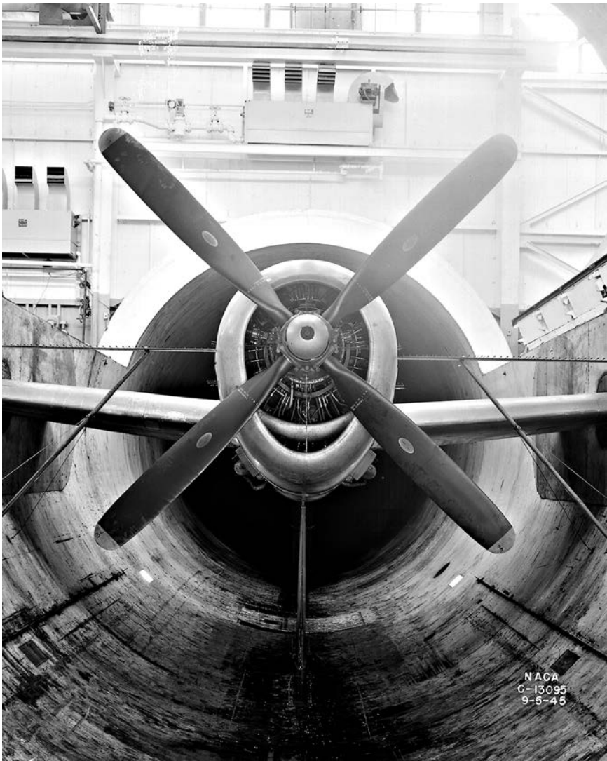
Shown above is a Republic XP-47M Thunderbolt fighter, complete with Hamilton Standard propeller and Pratt & Whitney radial engine, installed in the Altitude Wind Tunnel at the Aircraft Engine Research Laboratory in September 1945. (NACA)
