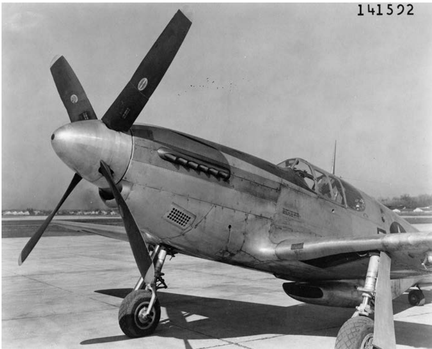
Figure 1-2. The use of propeller cuffs on fighters like the P-51 Mustang maximized the aircraft's overall performance. (National Air and Space Museum, Smithsonian Institution, NASM 7A35592)
