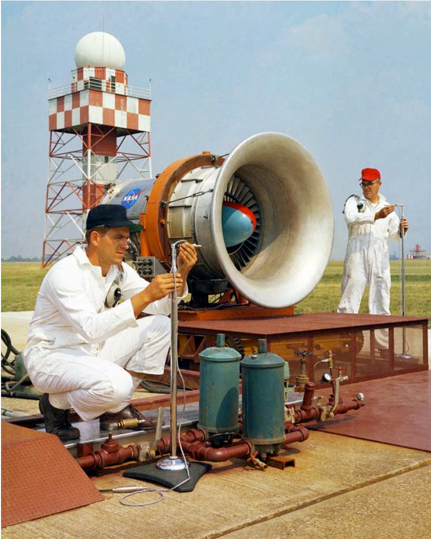
NASA technicians prepare for a jet engine noise test on the airfield at Lewis Research Center in 1967. (NASA)
