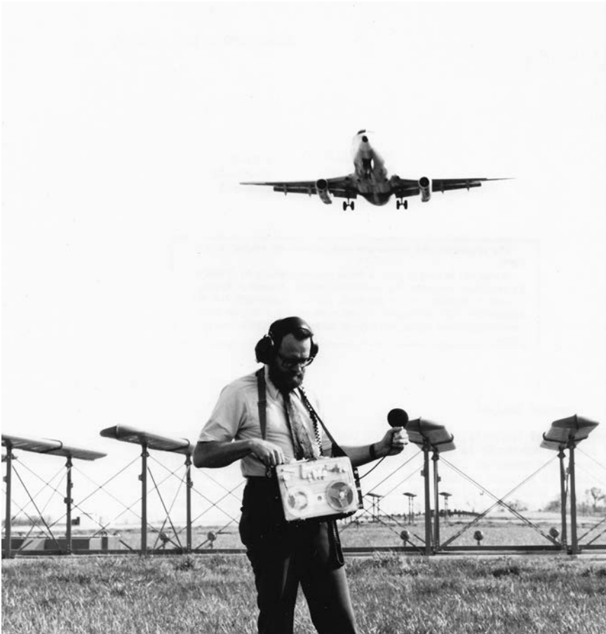
Figure 3-1. A researcher takes aircraft noise readings as part of an airport environmental control study. (NASA)
