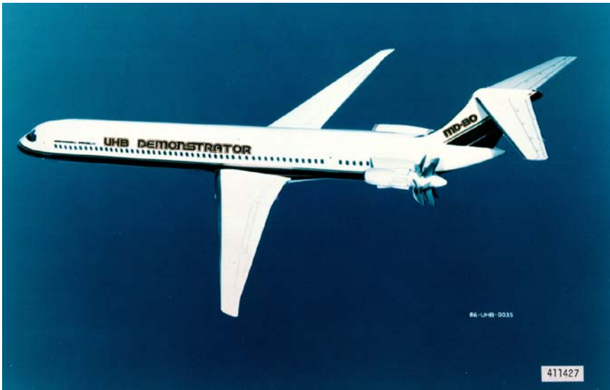
Figure 4-8. The McDonnell Douglas MD-80 UHB Demonstrator is shown with the 578-DX engine. (NASA)
