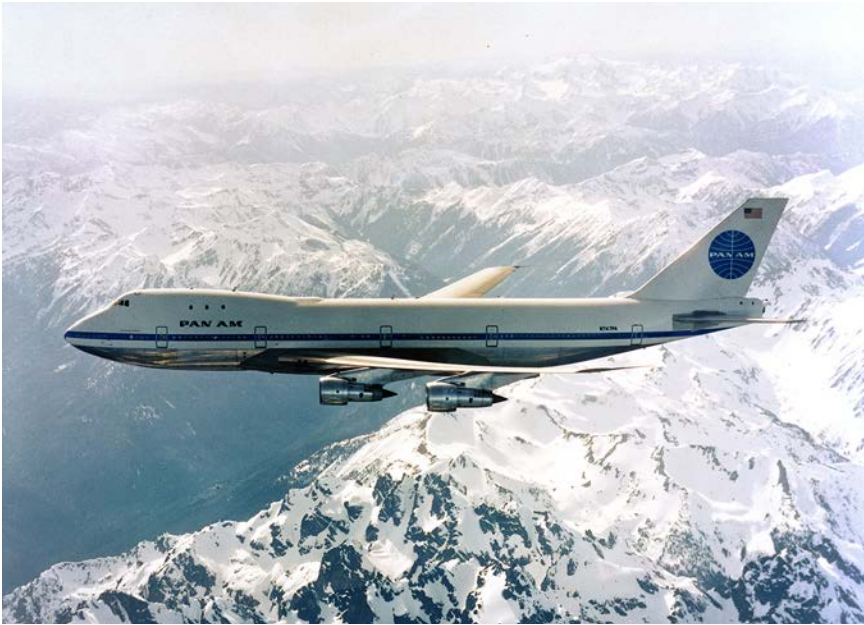
Figure 4-3. The high-bypass Pratt & Whitney JT9D powered a new generation of airliners, including the Boeing 747 jumbo jet. (NASA)
