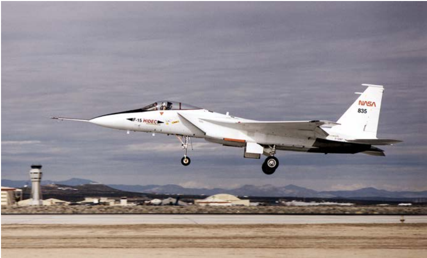
Figure 5-6. Gordon Fullerton uses only engine power to land the NASA F-15 at Dryden on April 21, 1993. (NASA)
