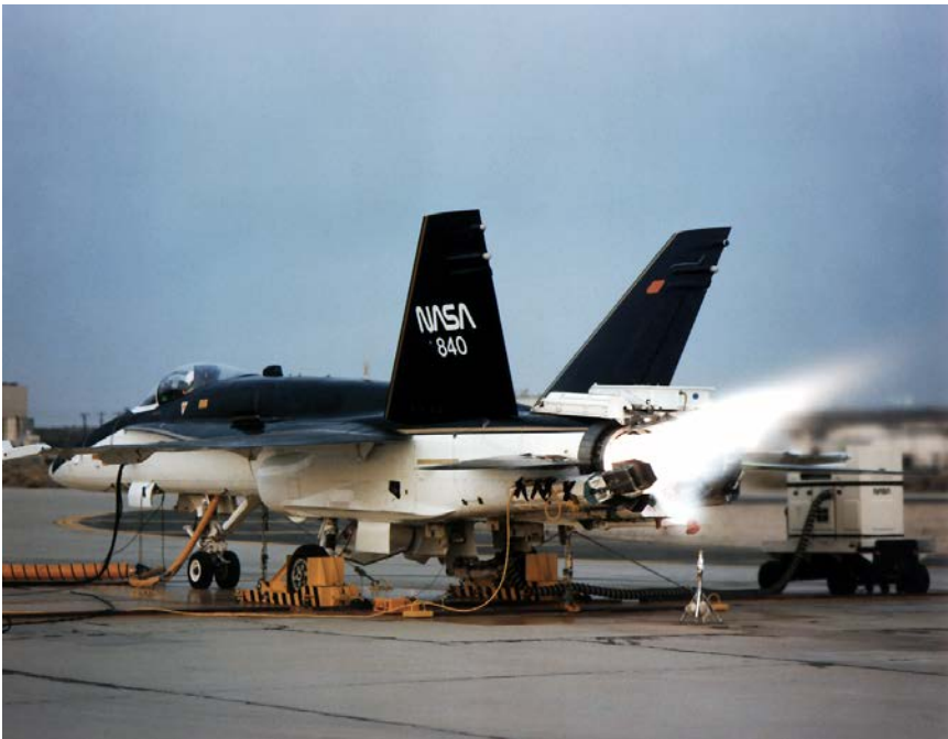
Figure 5-8. The use of thrust vectoring in the HARV program was an important precedent for later programs. (NASA)
