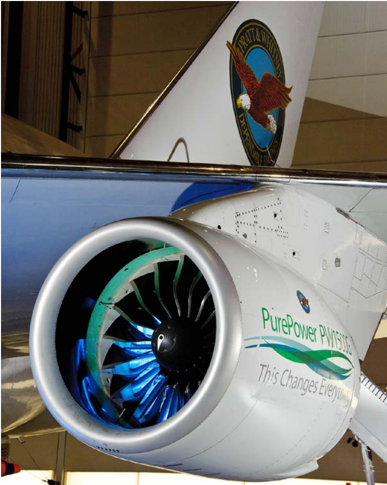
Figure 7-3. Pratt & Whitney's Geared TurboFan technology became the basis for the PurePower engine series. (Pratt & Whitney)
