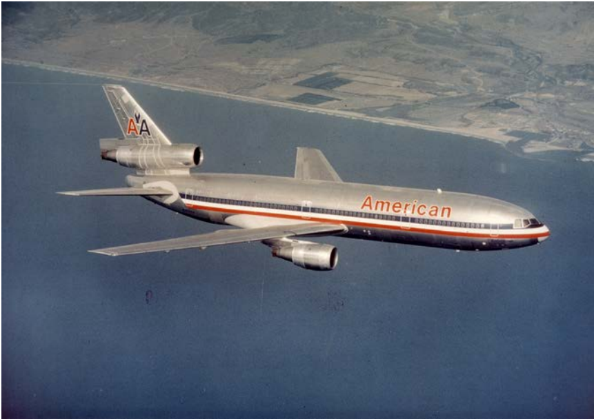
Figure 4-1. Three General Electric CF6 engines powered the McDonnell Douglas DC-10. (Boeing)
