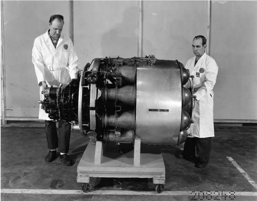
Figure 1-11. This image shows America's first jet engine: the General Electric I-A Engine. (National Air and Space Museum, Smithsonian Institution, NASM 9A11739)
