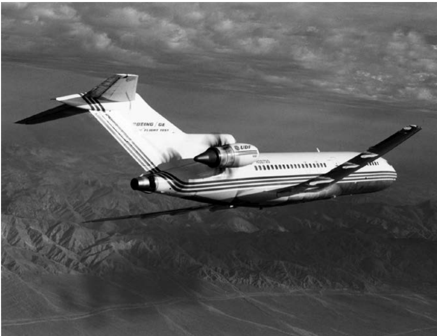
Figure 4-5. This image shows the GE36 UDF installed on the Boeing 727 demonstrator for flight tests. (National Air and Space Museum, Smithsonian Institution, NASM-9A11738)
