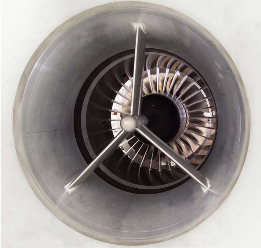
Shown above is an inlet view of a proof-of-concept two-stage compressor evaluated during the Ultra-Efficient Engine Technology Program at Glenn Research Center in 2005. (NASA)
