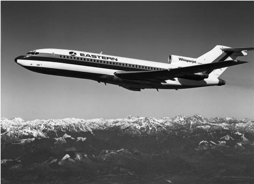
Figure 4-2. The Boeing 727 featured three Pratt & Whitney JT8D turbofans. (Boeing)
