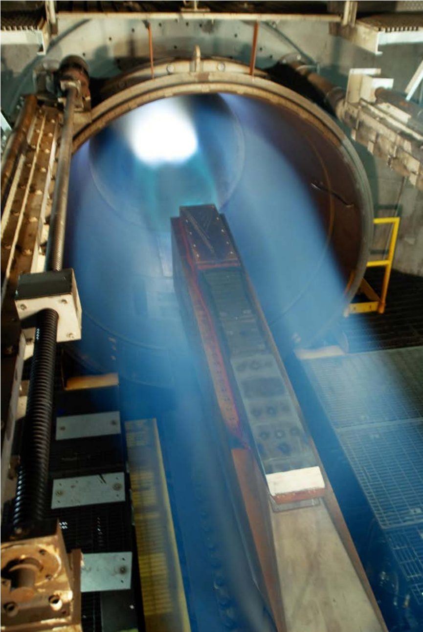
Figure 6-6. The Pratt & Whitney Rocketdyne SJX61-2 scramjet undergoes ground testing simulating Mach 5 flight conditions in the Langley 8-Foot High Temperature Tunnel. (NASA)
