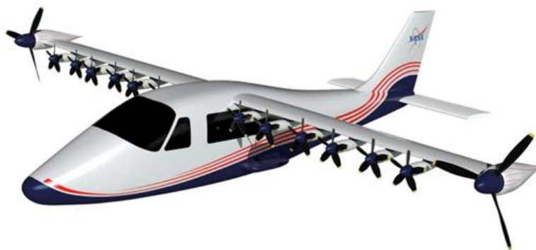
Figure 1. NASA X-57 Distributed Propulsion All-Electric Flight Demonstrator.
