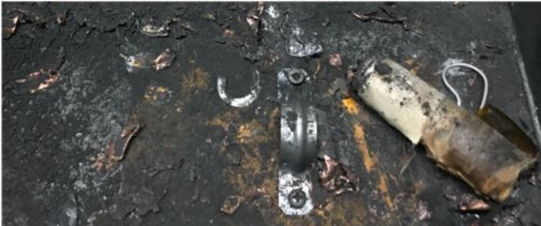
Ambient thermal runaway first vented and then flared up leaving black residue.
