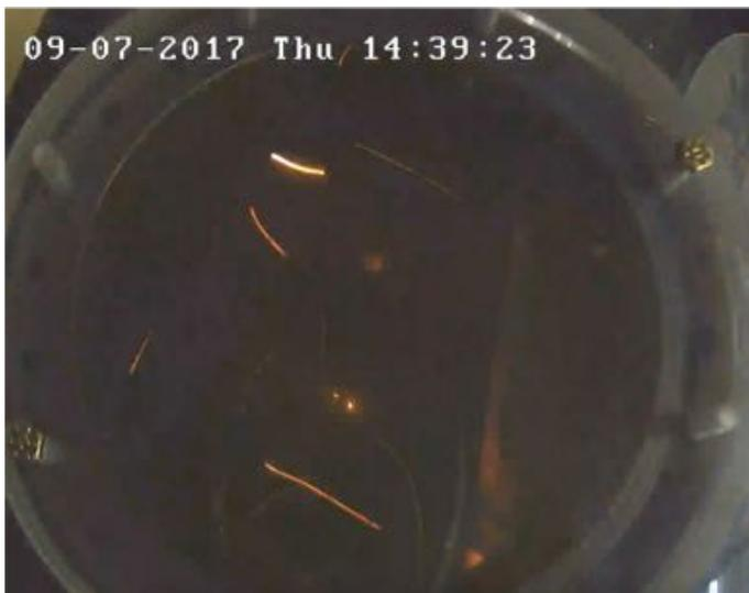
Ignition following the venting of the cell. Ignition event lasted ~1.5 s. After event, thick gray/black particulate obscured viewport.
