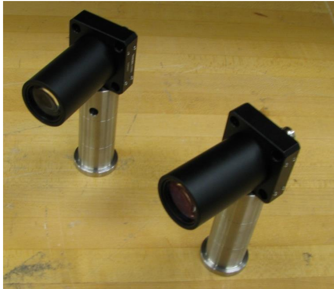
Figure 6. Two haze receivers, composed of a lens and large-area photodetector
