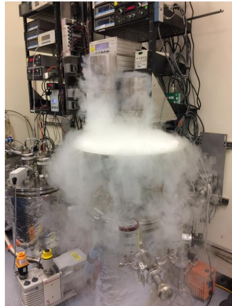
Figure 2. Cryostat-500 during test specimen installation (left) and cooldown operation (right).
