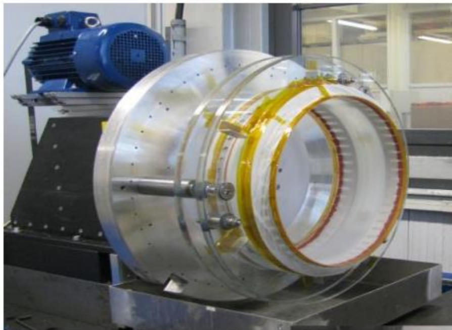
Figure 1. Photograph of a 2-mm thick, 486.5-mm diameter full-shell fused silica optic mounted on a fixture developed by Brera/INAF [credit: Brera/INAF].
