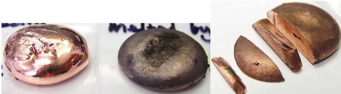
Figure 1.—As-received, ~1-in.-diameter ingots of pure Cu (left) and Cu-0.4C (wt%) before washing (center). Both ingots were covetically processed. The Cu-0.4C ingot after washing and cutting is shown (right).
