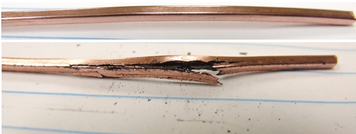
Figure 4.—Hot isostatically pressed and rolled pure Cu sample (top) and Cu-0.4C (wt%) (bottom). In both cases, the sections were HIPed as is, without being placed in a copper tube prior to HIPing; the lines on the paper are 7 mm apart.
