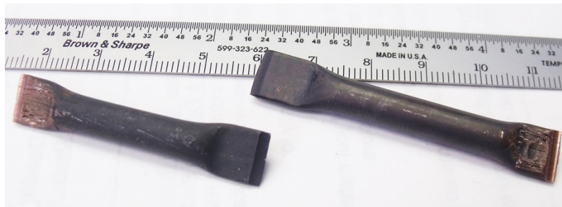
Figure 3.—Samples sealed in evacuated, pure Cu tubes.
