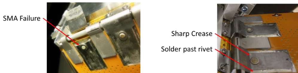
Figure 6. SMA Hinge Spring Failed Flight Attachment
