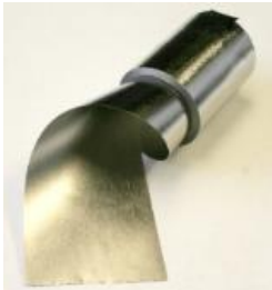
25-mm by 1.6-km spin cast ribbon
