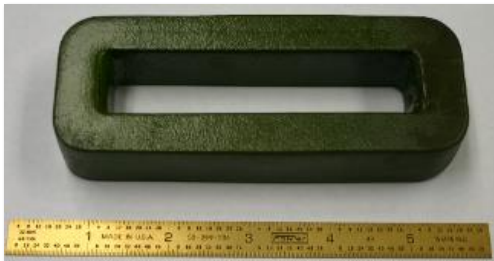
Transformer fabricated from spin cast ribbon
