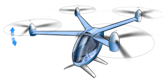
Figure 1. Single-passenger quadrotor with electric propulsion.
