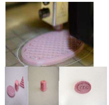
FDM prints using reclaimed anti-static bagging film with reversible cross-linking additive (image from Cornerstone Research Group)
