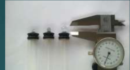
3, 5, and 8 mm particles adhered to interchangeable plungers
