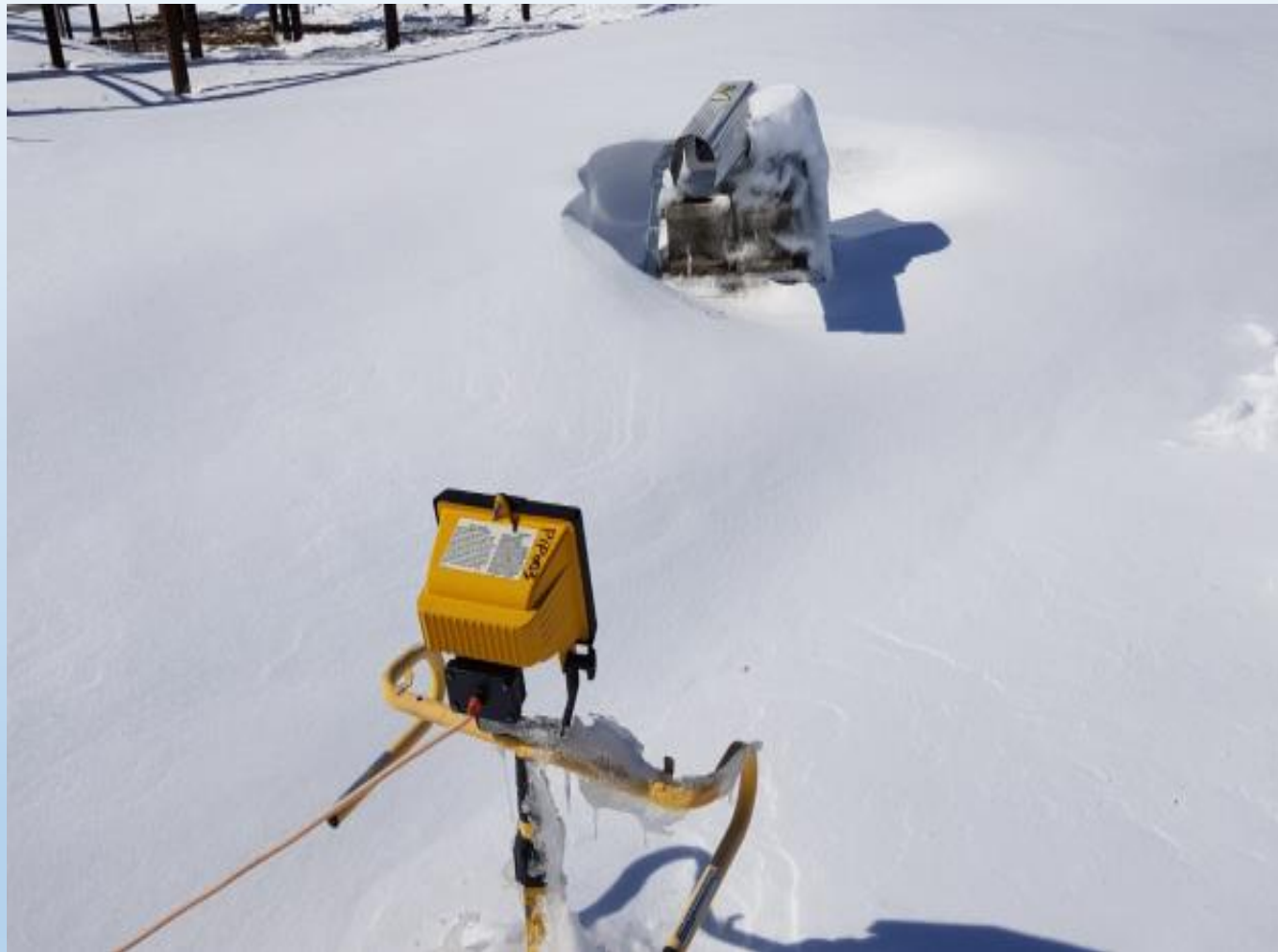
NASA Precipitation Imaging Package (PIP; left) and PIP observations of 2.5+ cm diameter snowflakes, associated with 28 February snowstorm ( courtesy: Kwonil Kim, KNU )
