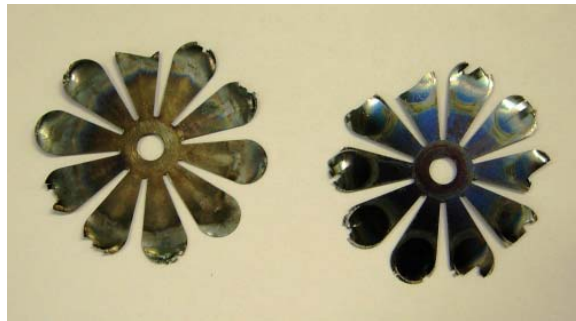
1950's era RPC Reed Valves After 15 sec. Operation in Gas Turbine
