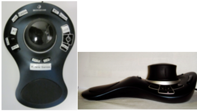
Figure 2. The Connexion SpaceExplorer input device used to control the UAV payloads/sensors.
