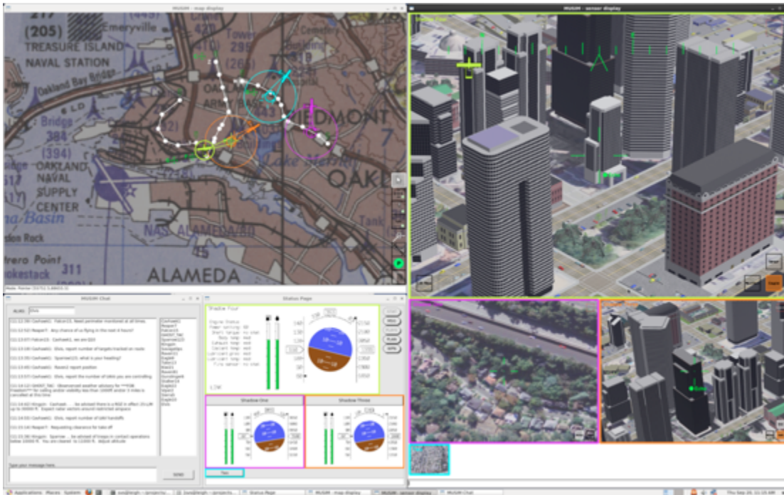
Figure 7. Two UAVs (outlined in the lime [upper payload window] and orange [middle right payload window]) coupled together sharing the same stare point and loiter waypoint.
