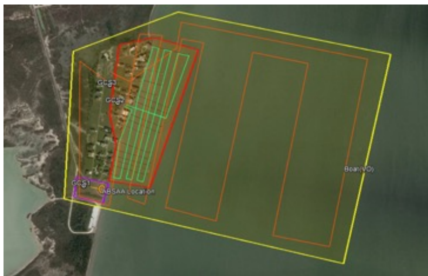
Figure 3. Example objective-specific scenario, designed to use altitude-stratified operations, BVLOS operations, and altitude-stratified BVLOS operations to investigate responses to alerts from the UTM system and airborne surveillance/sense and avoid.
