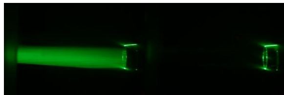
Figure 6 – Electrostatic precipitator off (left) and electrostatic precipitator on (right) indicating a high level of dust clearing efficiency
