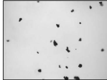
Figure 5 – Sample image of approximately 50 µm diameter particles
