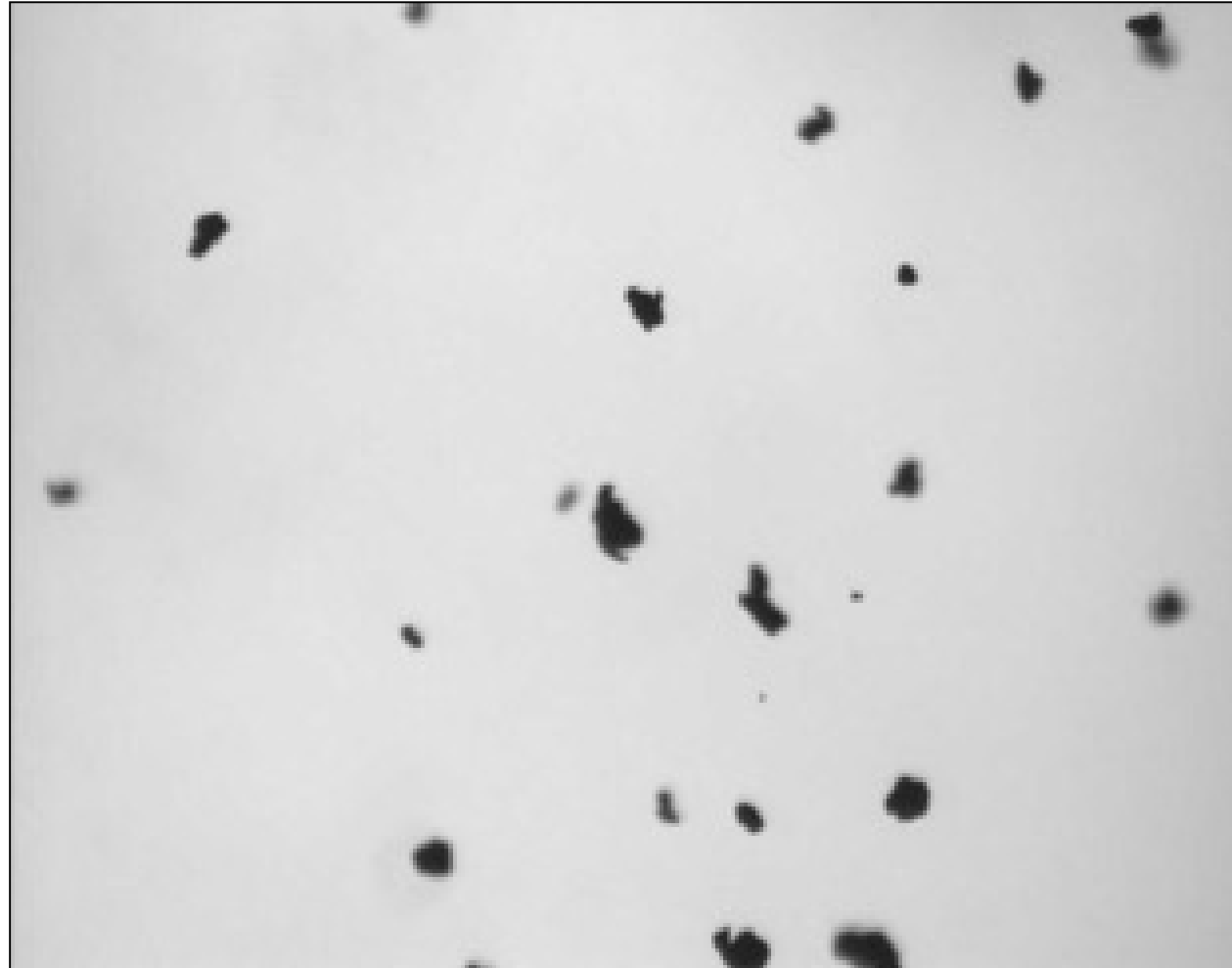
FPA sampling 50 \mu\text{m} diameter particles in ESP testbed
