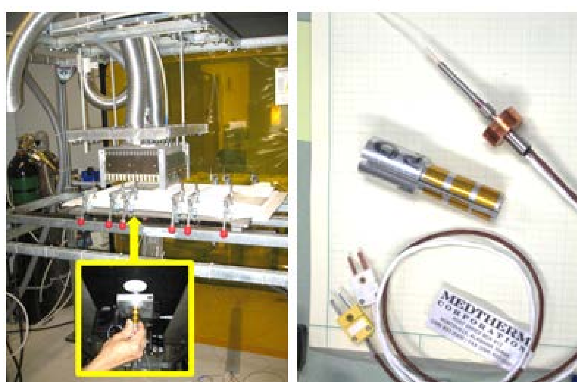
High-temperature sapphire rod coupled to mini-spectrometer configuration was tested using NASA Quartz Lamp source. Plots shown give effect of sapphire rod on system response and a representative calibration using integrating sphere. (Cruden & White)
