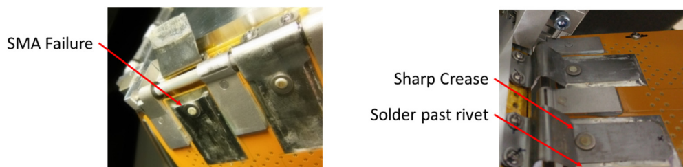
Figure 6.—SMA Hinge Spring Failed Flight Attachment.
