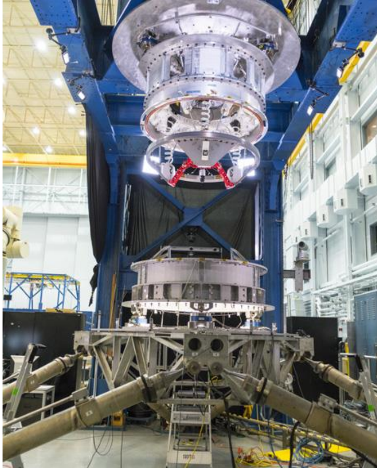
Figure 8. NDS 6DoF Docking Test
