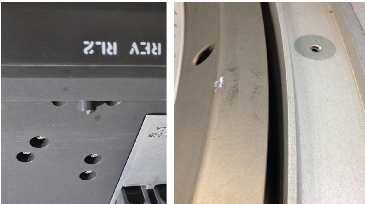
Figure 14. Capture sensor and opposing ring wear pattern during development testing
