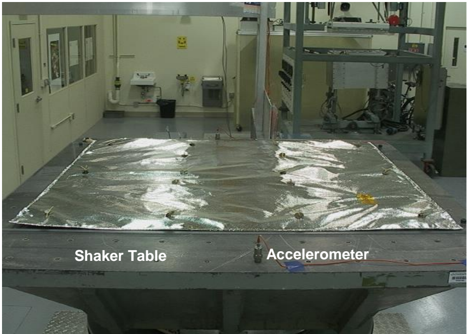
Figure 2. Shaker table experiment with aluminized MLI blanket.
