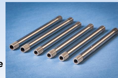
NiTiHf Shape Memory Alloy torque tube actuators for UAV
