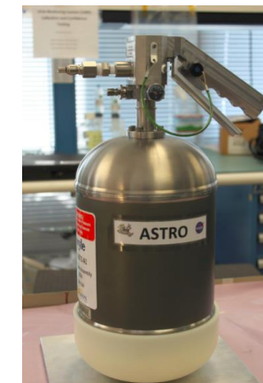
Engineering Development Unit of an ISS FWM PFE
