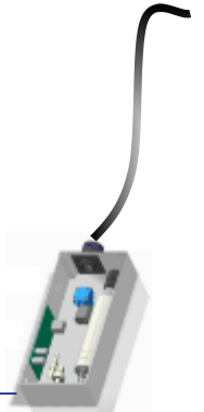
Remote Sensors (6) Measure temp & CO_2 in standoffs, hatch and end cone
