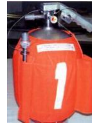
US CO 2 fire extinguisher
