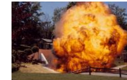
Coal dust test explosion
