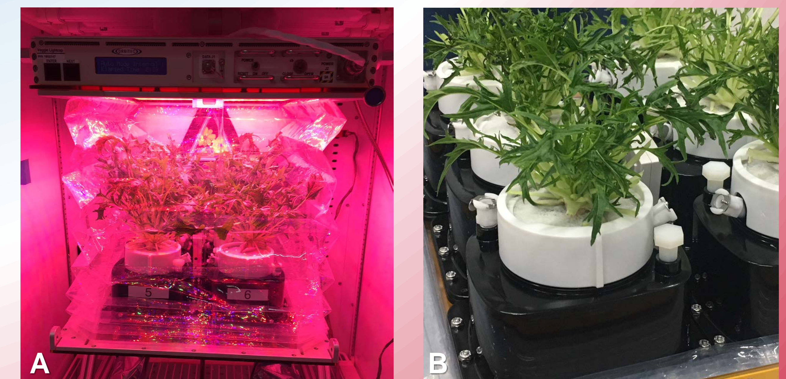
Fig. 7 A. Mizuna plants growing in Veggie in the PONDS hardware during the VEG-04 SVT. B. Close up of PONDS units after 1 st cut-and-come-again harvest.
