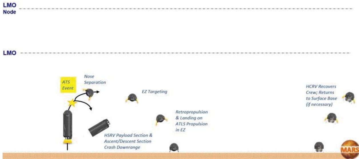
Figure 13. Concept of operations illustrating Mars ascent ATS targeting a return to exploration zone using the ATLS propulsion system only.
