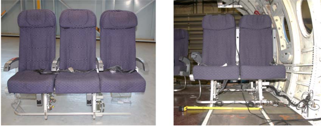
Figure 7 - Double seat configuration for port side. Unmodified triple (left) cut and modified into a double (right)
