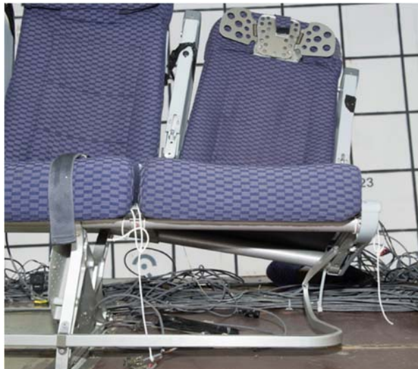
Figure 40 - Post-test rear triple aisle seat deformation (seat 3)
