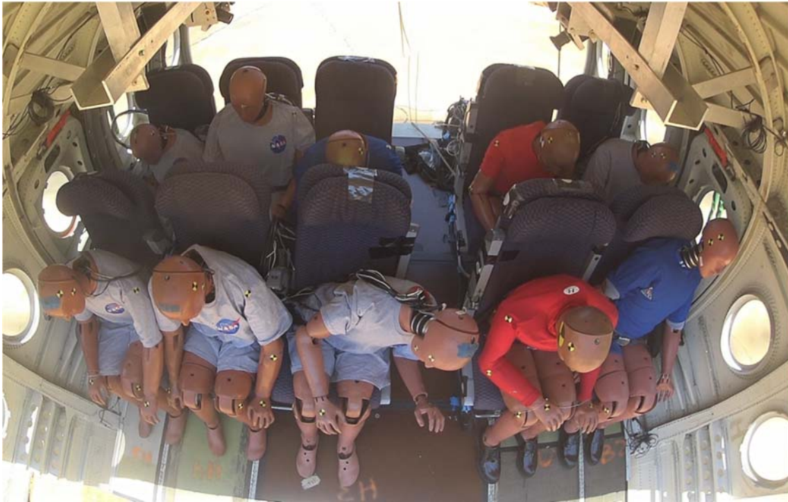
Figure 71 - Wingbox Section post-test ATD positions
