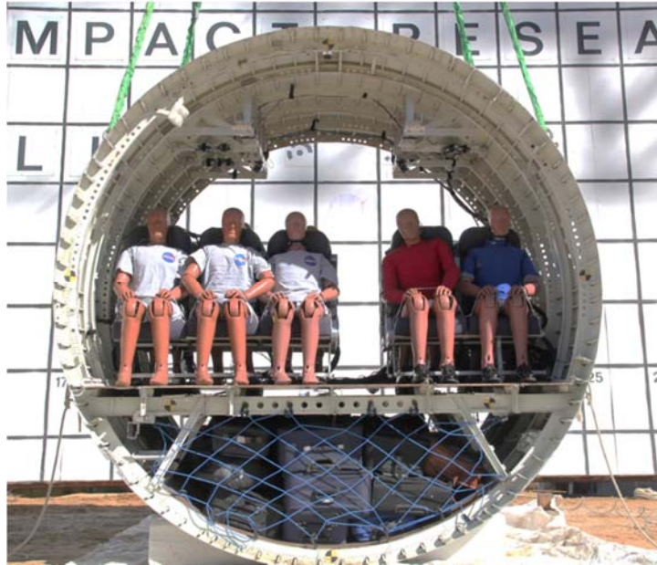
Figure 14 - Forward Section test article
