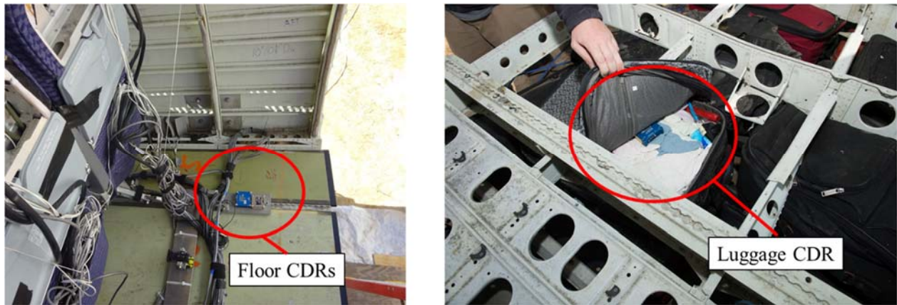
Figure 12 - Forward Section CDRs. Floor level (left) and luggage (right)
