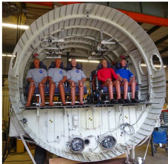
Figure 15 - Wingbox Section test article
