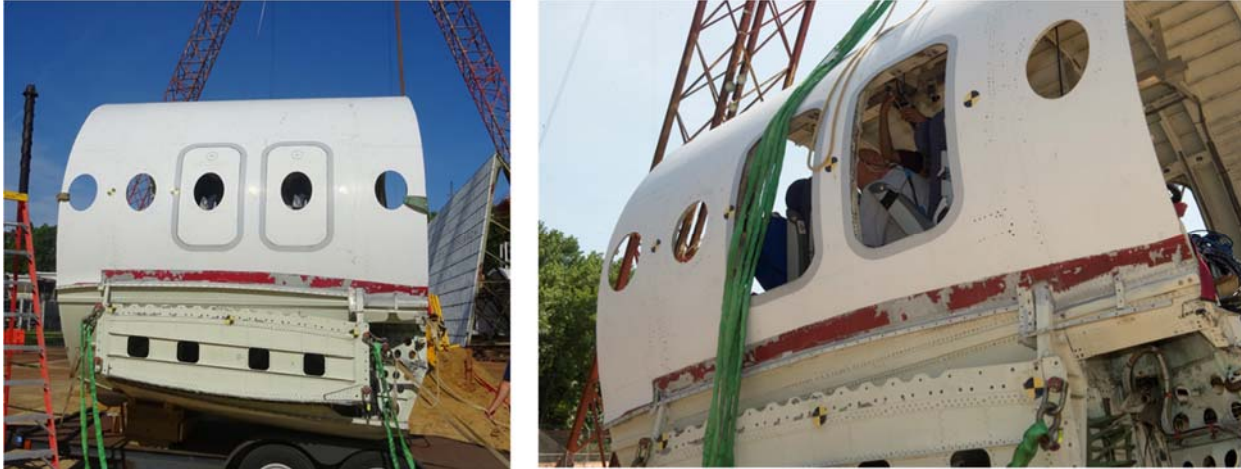
Figure 52 - Wingbox Section port emergency exit doors pre- (left) and removed post-test (right)
