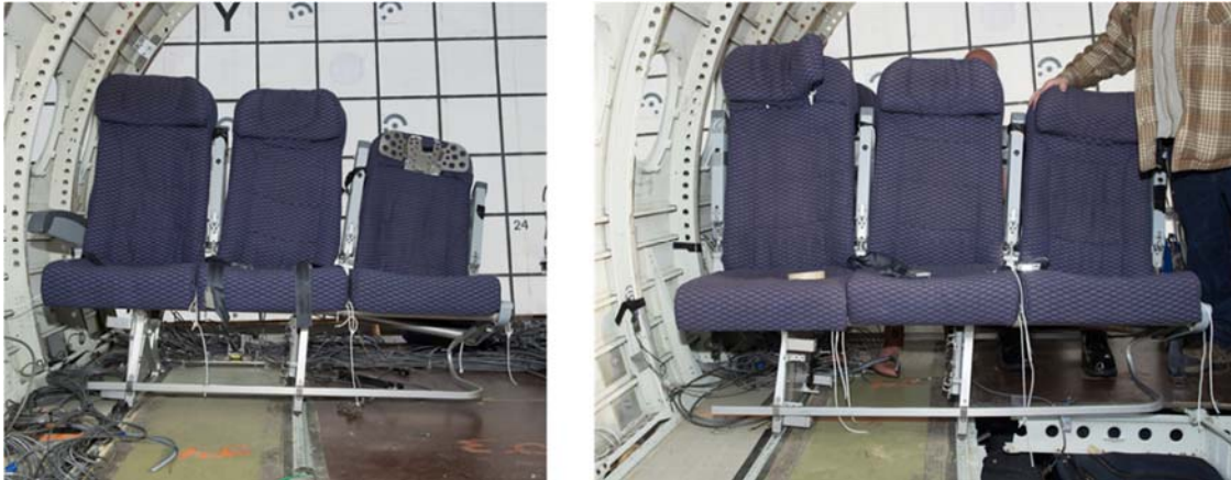
Figure 39 - Post-test triple seats. Rear (left) and front (right)
