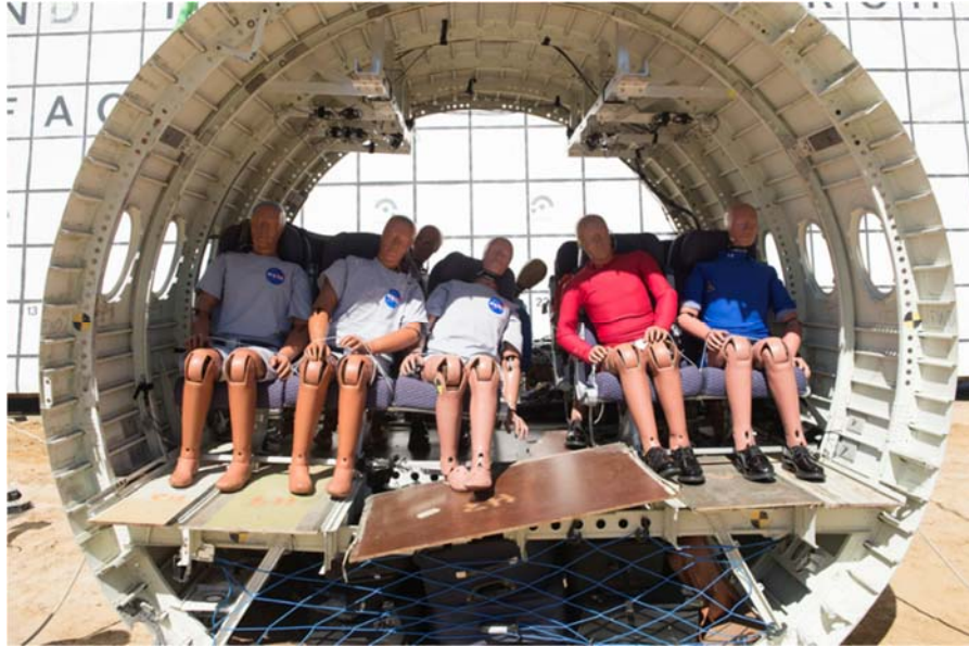
Figure 34 - Forward Section front row ATDs (Seats 6 through 10)
