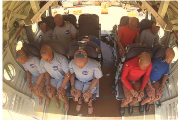
Figure 10 - Seat schematic (left) and picture of ATDs in test configuration (right)
