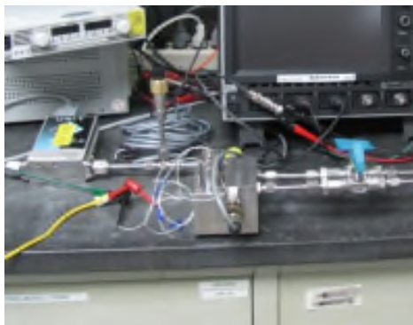
Figure 12: MFC Bench Unit in Test (left) and Closed Loop Pressure (Flow) Response (right)
