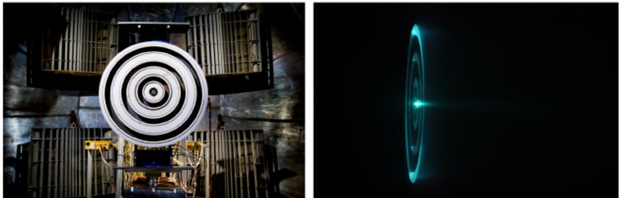
Figure 6. Photographs of X3 installed in University of Michigan's LVTF (left) and operating three channels simultaneously at 30 kW (right).
