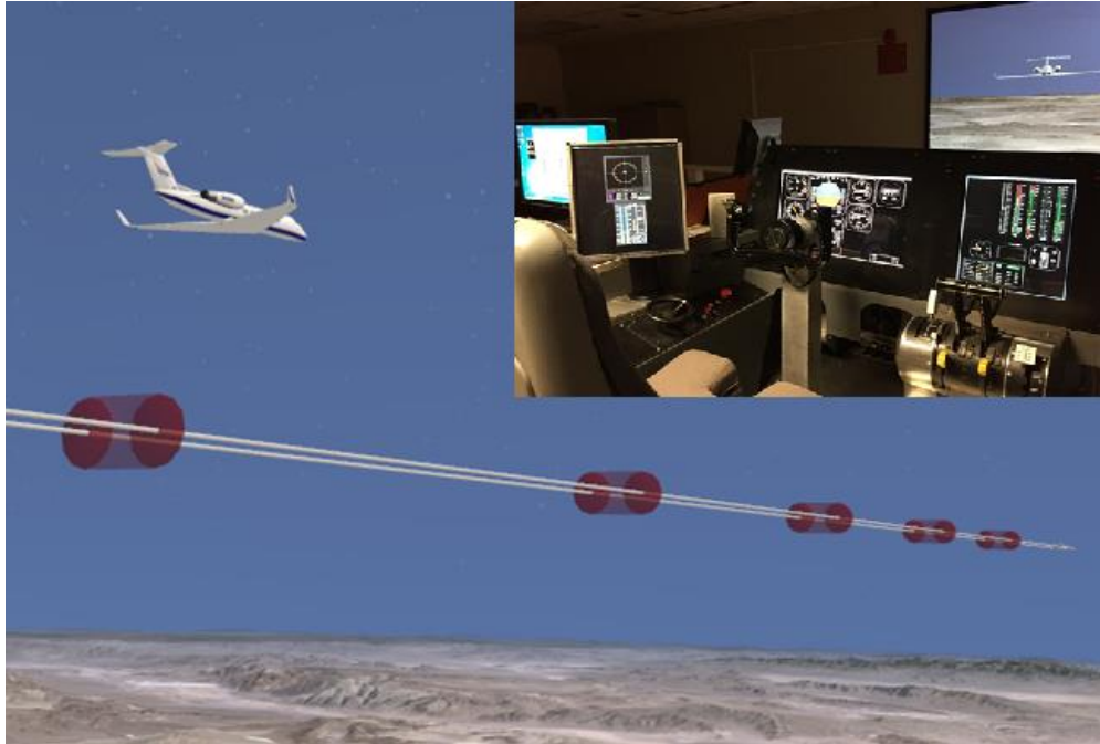
Fig. 5. Simulation display of the G-III airplane with the wake vortex model and pilot simulation setup.
