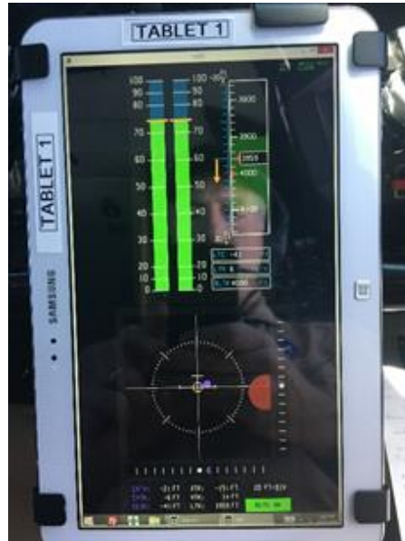
Fig. 14. Long-track and wake awareness display running on pilot tablets during a wake surfing experiment.
