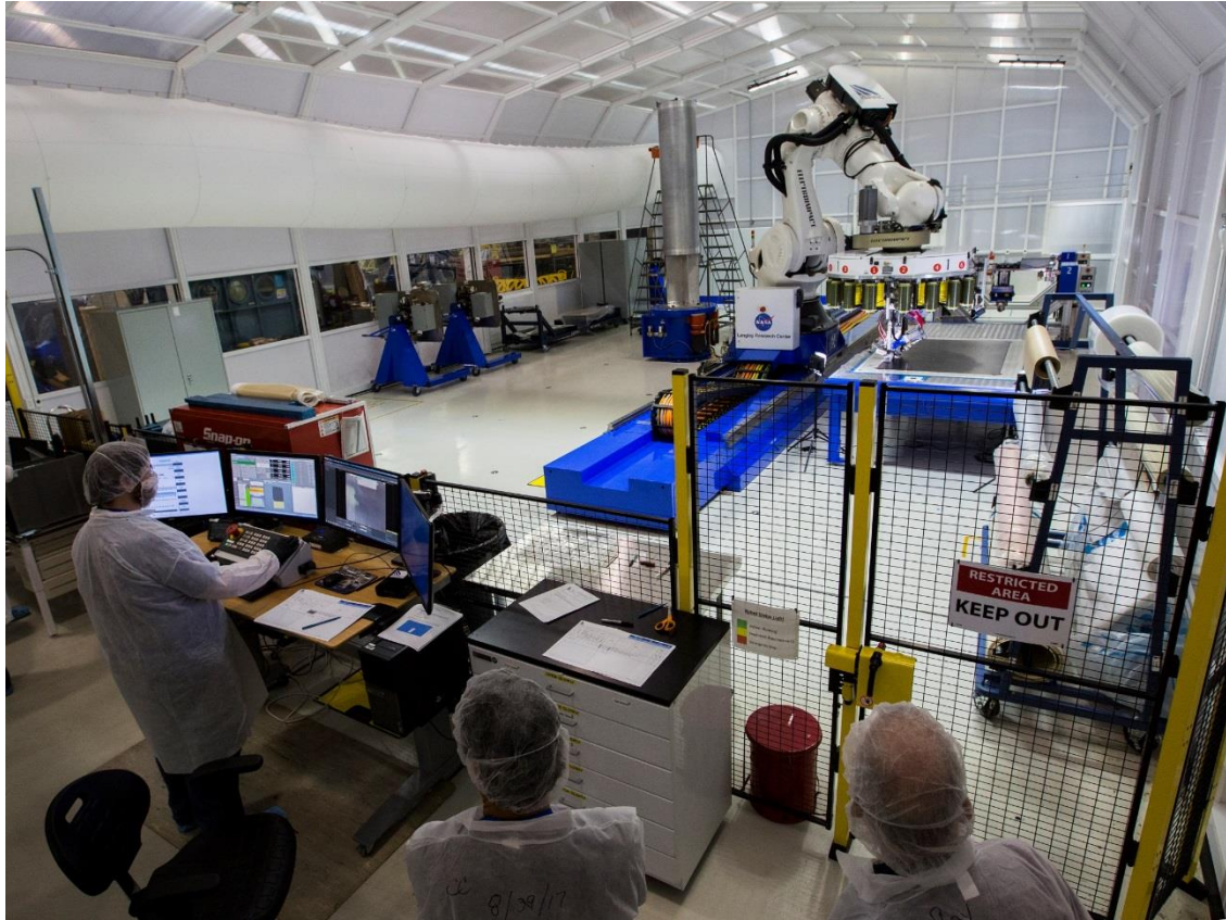
Figure 1: Equivalency panel fabrication with the ISAAC robot at LARC.
