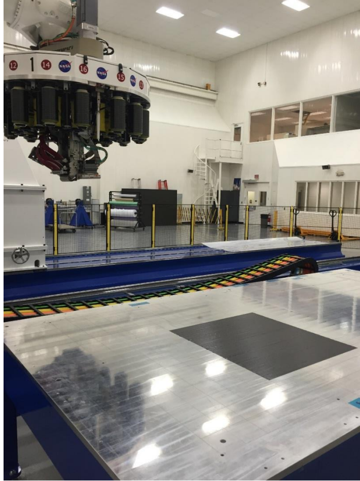
Figure 2: Equivalency panel fabrication at MSFC.
