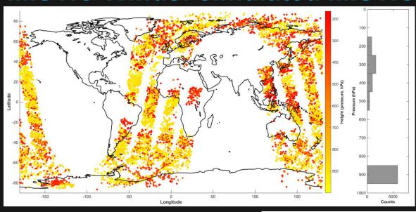
➤ Considering only one orbital plane (3 satellites), MISTiC Winds is able to collect approximately 13,000 cloud AMV observations and 5,000 water vapor AMVs every 6 hours.
