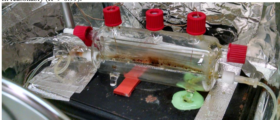
Figure 9. End of V-tube run showing sever discoloration of the DGA as well as condensing DGA inside V-tube
