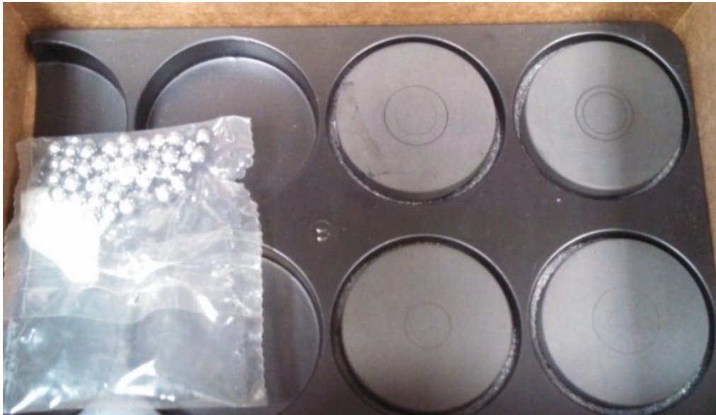
Figure 5. Test Specimens for low speed wear testing
