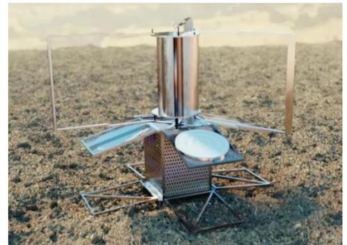
**Fig. 1** Notional wind powered version of the Long-Life In-situ Solar System Explorer Venus Probe Concept
