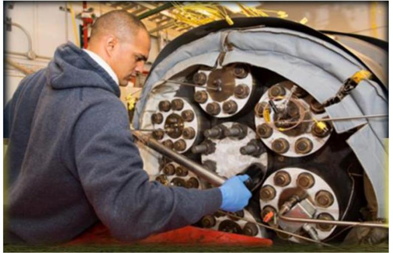
**Fig. 2** Testing in GEER at Venus surface conditions
