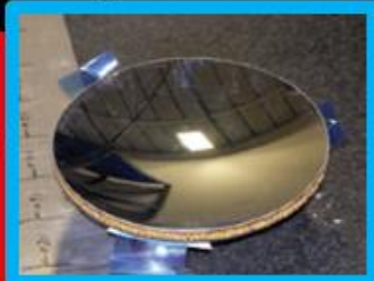
Composite primary optical reflector
