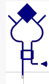
Initial 20 GHz Microstrip Patch Feed (length is 0.620")
