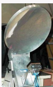
WISM reflector antenna with WISM antenna feed
