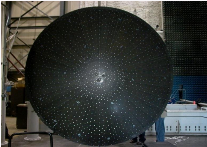
Composite Technology Development 3.2 m Shape Memory Polymer Composite Reflector at GRC Near Field
